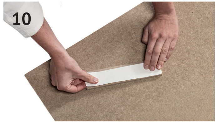
10 Press firmly to stick the double sided tape to the felt spacer
