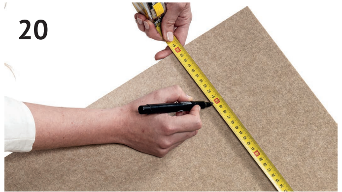
Mark a dot 10 centimeter from the upper edge on the right side
