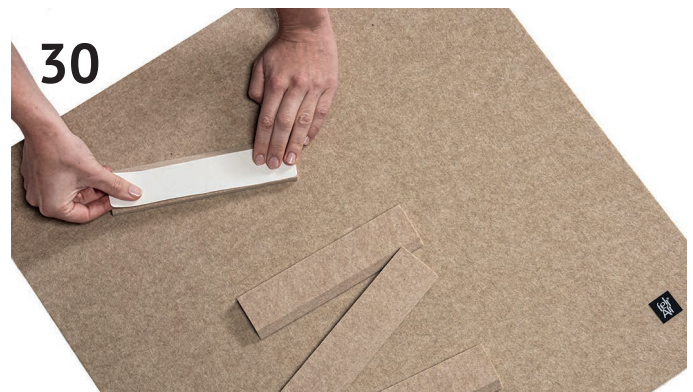
30 Press firmly to stick the double sided tape to the felt spacer
